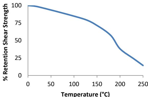
"Hot strength" shear strength. Fully cured specimens conditioned to pull temperature for 30 minutes before testing at temperature.
