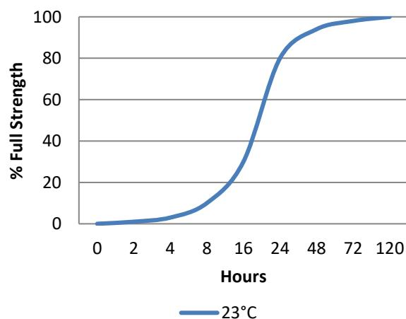
Graph shows typical strength development of bonded components. An increase of 8°C in temperature will halve the cure time. Lower temperatures will result in a slower cure time.
